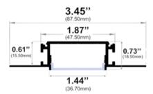
Width (outside): 1.44" (36.70mm) Width (inside): 1.18" (30.00mm) Height: 0.61" (15.50mm) Length: 94" (2.38m)
