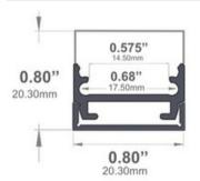
Width (outside): 0.80" (20.30mm) Width (inside): 0.68" (17.50mm) Height: 0.80" (20.30mm) Length: 94" (2.38m)
