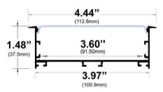
Width (outside): 4.44" (112.8mm) Width (inside): 3.60" (91.50mm) Height: 1.48" (37.50mm) Length: 94" (2.38m)
