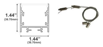
Width (outside): 1.44" (36.70mm) Width (inside): 1.18" (30.00mm) Height: 1.44" (36.70mm) Length: 94" (2.38m)
