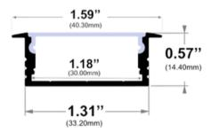
Width (outside): 1.31" (33.20mm) Width (inside): 1.18" (30.00mm) Height: 0.57" (14.40mm) Length: 94" (2.38m)
