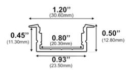
Width (outside): 1.20" (30.60mm) Width (inside): 0.80" (20.30mm) Height: 0.50" (12.80mm) Length: 94" (2.38m)
