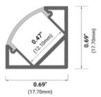
Width (outside): 0.69" (17.70mm) Width (inside): 0.47" (12.10mm) Height: 0.69" (17.70mm) Length: 94" (2.38m)
