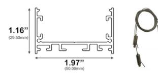
Width (outside): 1.97" (50.00mm) Width (inside): 1.80" (45.72mm) Height: 1.16" (29.50mm) Length: 94" (2.38m)
